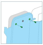
Slide the payment device as shown, and secure via the (4) included screws.
