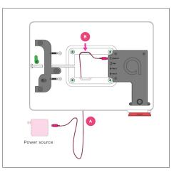
**A.** Feed the provided Anker USB-C power cable through the kiosk and plug it into a power source. **B.** Route the Anker USB-C power cable through the cable paths and plug it into the port labeled "Power In."
