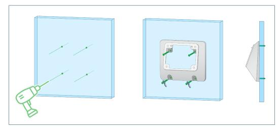
\*Aila provides hardware for securing to studs and drywall. For all other surfaces, choose an appropriate #10 fastener.
