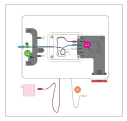
C1. Plug the Apple-provided USB-C cable into the port labeled "iPad."C2. Secure the other end of the Apple-provided USB-C cable along the left-side cable path and beneath the strain release (small black tab). Close the strain release, securing the cable (shown in green). D. If you have accessories, use Port 1 & 2. Secure your cable(s) with the bottom cable path.
