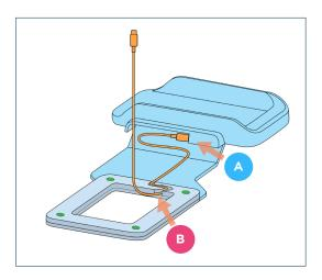
Plug the Micro-USB end of the supplied power cable into socket (A) on the payment cradle.
