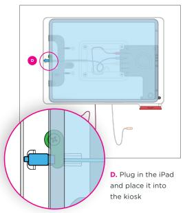
**DETAIL:** Apple USB-C plug flips up and over to fit flush between the iPad and Kiosk wall.
