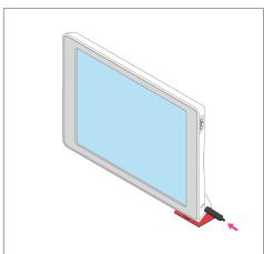
To power-on the iPad, use the provided access key fob to press the power button on the lower right side of the kiosk.
