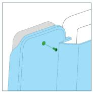
Slide the payment device as shown, and secure via the included screw.
