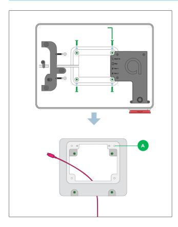
Orient the Kiosk enclosure with the Kiosk mounting holes (A), and fasten it with the supplied wrench and flat head screws.
