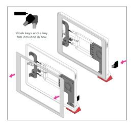
On the back of the unit, insert the kiosk key into the barrel lock and twist to unlock the front panel. Remove the faceplate from the kiosk by pulling the left side of the plate first, and then unhooking the right side. Remove the kiosk key from the back of the kiosk.
