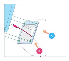
Plug the Micro-USB end of the supplied power cable into socket (A) on the payment cradle.
