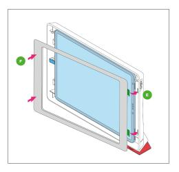
**E.** Reattach the faceplate right (or "hooked") side first. Slide the tabs into the enclosure, and firmly press down on the left edge (F) to fully engage the latch. **TIP:** be sure to remove the kiosk key from the back of the kiosk before securing the faceplate.
